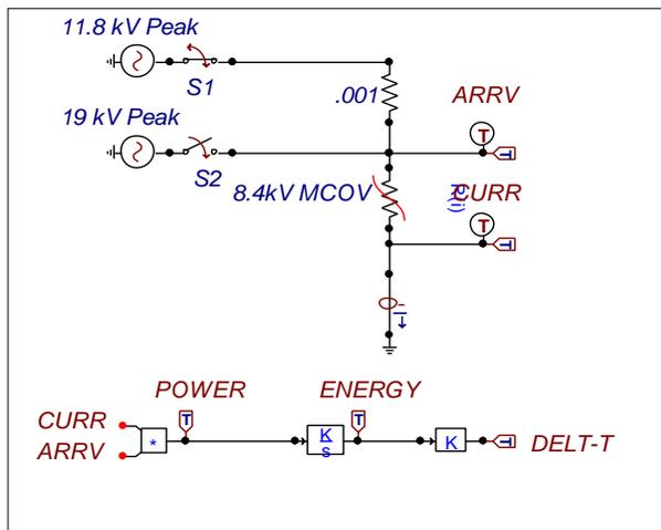
**Figure 4:** 60 Hz Overvoltage Stress of an arrester that generates a temperature rise.
