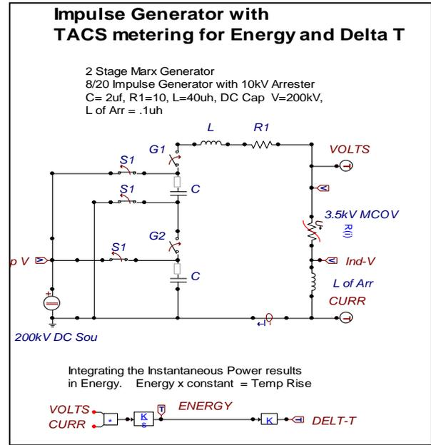
Figure 2 ATP Model of an Impulse Generator with TACS metering of Arrester
