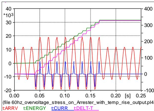
**Figure 5:** 60 Hz Overvoltage Stress of an arrester that generates a temperature rise. ARR and ENERGY referenced to Left Y axis.
