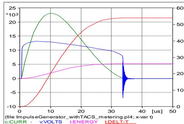
Figure 3 Plot of Temperature Rise from an Impulse Arrester Current, Voltage and Absorbed Energy on the left Y axis and Delta T in °C on the right Y axis
