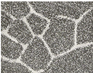
Figure 5 Microstructure of ZnO element
