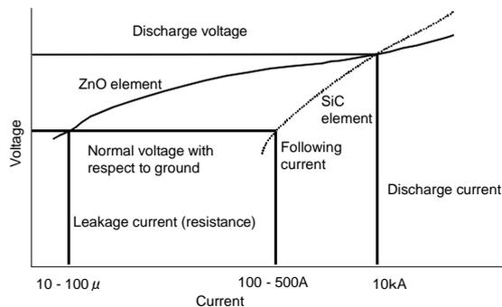
**Figure 3 Voltage vs. current performance of ZnO element**
