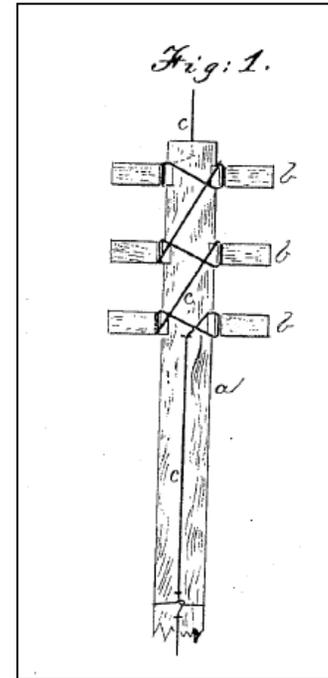
Figure 4 - Early Lightning Rod on Telegraph Pole
