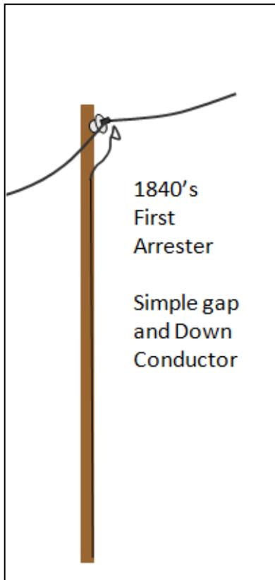
Figure 5 - Rendition of First Lightning Arrester 1850s
