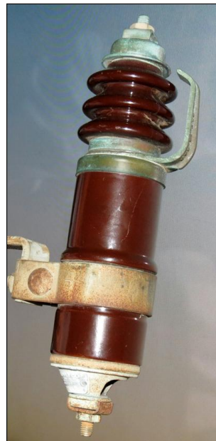
Figure 3a Early Expulsion Arrester by Joslyn Supply Co. 1940 Vintage
